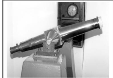
*The Transit Telescope at Orwell Park. This instrument was used to accurately determine local stars by their timed transit over the north/south meridian*
